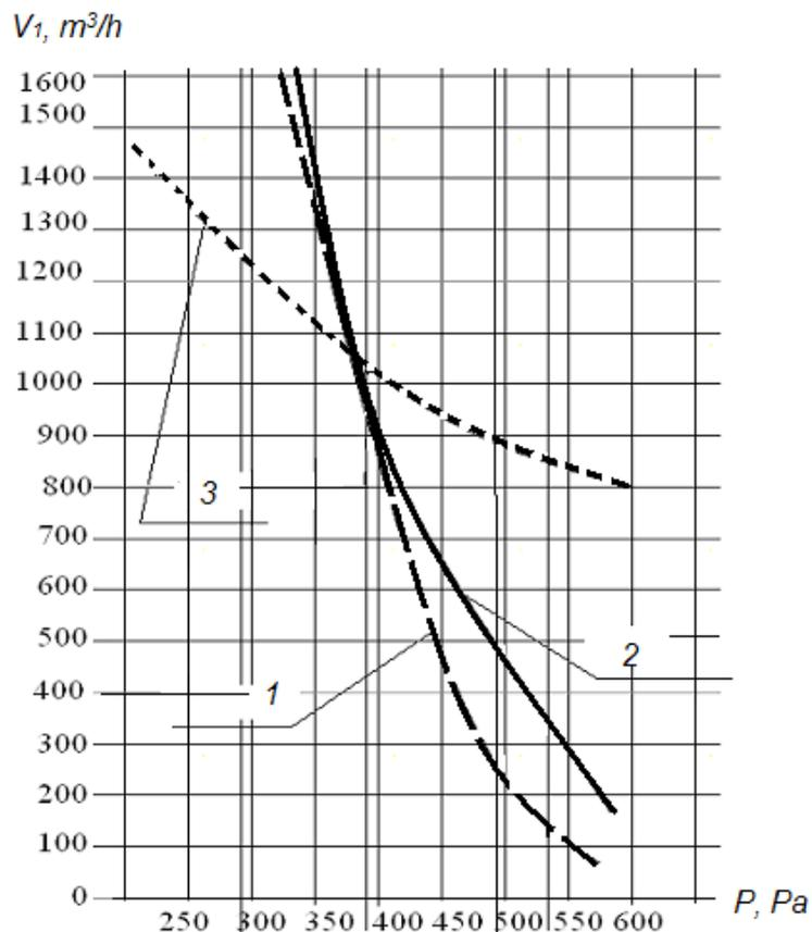
**Fig. 2.** Nomogram of required air exchange depending on cooling conditions to ensure  $C_d = MPC/2$
